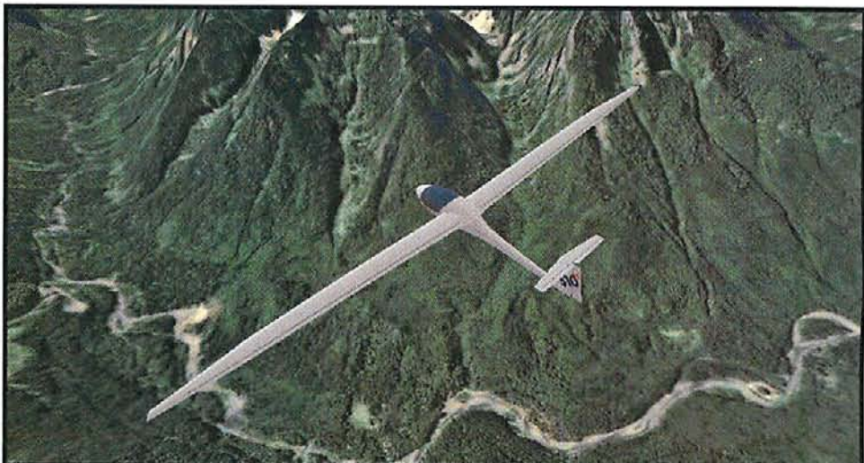
LOOK, MA, NO PROP The Stemme S10-VT glider has a retractable propeller, so it can take off and cruise to altitude under its own power.
